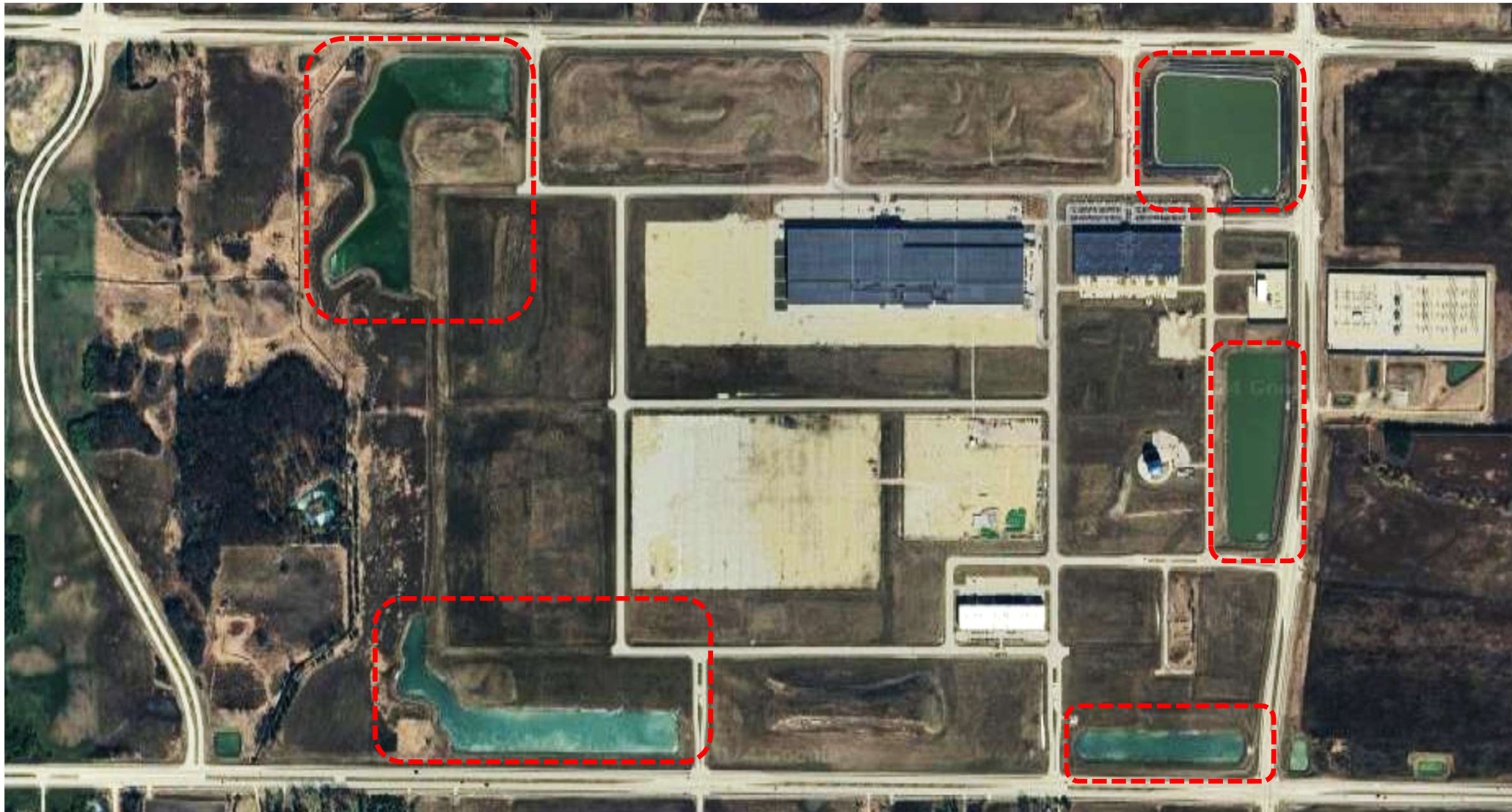
Plan view of the Foxconn/Microsoft campus showing the stormwater ponds that can be used for cooling the data center
