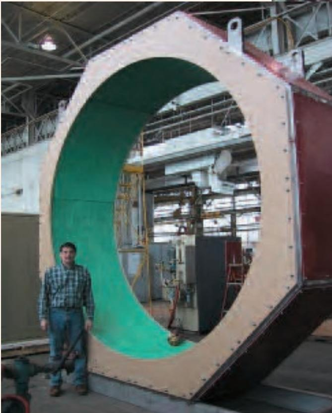
Close tolerance pipe coating with good bonding characteristics make induction heating the ideal method of pre-heating line pipe. Equipment is available to handle a wide range of pipe sizes.
