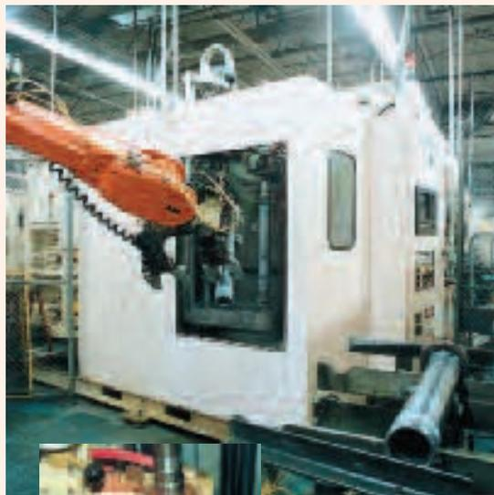
Robots load and unload heavy truck axle tube assemblies into a heavy duty single spindle vertical scanner for hardening and tempering.
