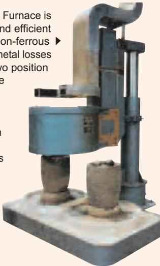
Magna-Melt Furnace is a rugged design for high frequency melting applications. Cast refractory top and bottom, stainless steel tie rods and the heavy-duty fabricated aluminum side plates form a rigid structure. ▼
