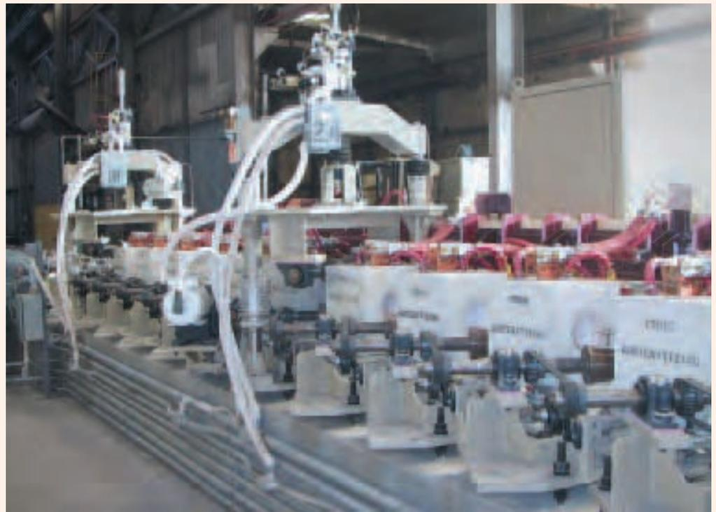
Ajax TOCCO quench and temper lines for solid bars and shapes are known industry wide for producing superior metallurgical and physical properties in the final product. These benefits are achieved with the ultra high heating rates and temperature control possible only with induction heating.
