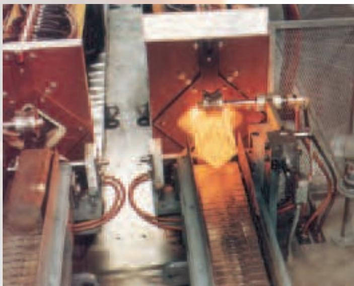
The first of several dual-line heaters supplied to process in excess of 12,000 pounds per hour.
