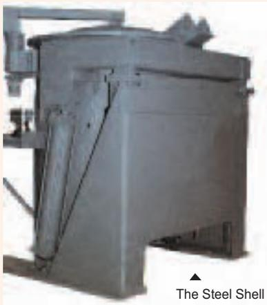
▲ The Steel Shell Furnace design provides maximum strength and support for all melting applications. Ideal for use with charge buckets and vibratory conveyor charge systems.
