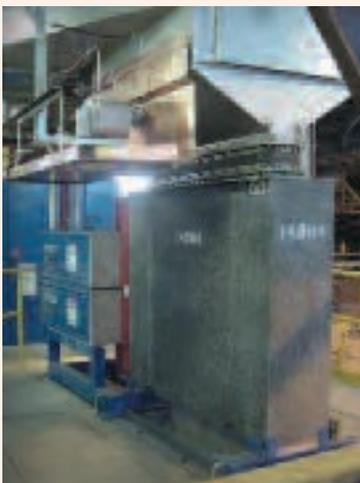
A view of a 1200 kW strip drying application. This equipment is being used for a wide variety of coating applications. The equipment is designed for horizontal or vertical installations.
