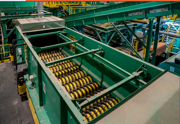
Size separation devices Full lineup of screens to remove oversized material, fines and organics.
