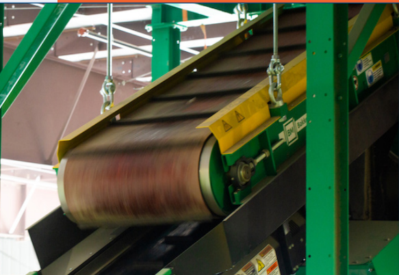
Metal separation Magnets and Eddy currents target ferrous and non-ferrous metals.
