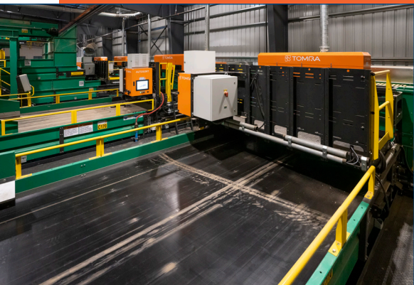
Optical sorting Separate containers by grade and sort plastics to make fuel products.
