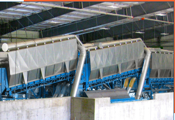
Density separation Separate good feedstock materials by density.
