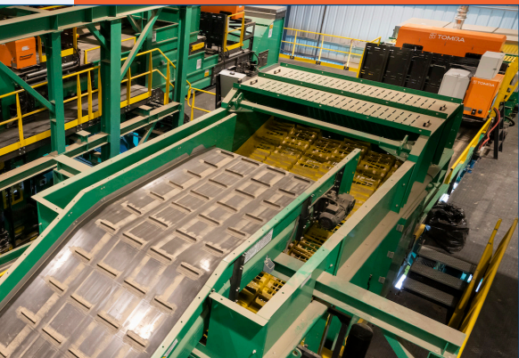
2D/3D separation Skim off 2D materials while screening out minus materials. No-wrap, no-star design.
